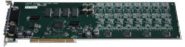
The configurable front-end of the CSE-8225 provides the user with a flexible solution for a wide range of applications. The gain for each channel can be individually set in a range of 1/4 to 4096 in steps of 2. Each channel also has configurable high pass and low pass filtering stages.
